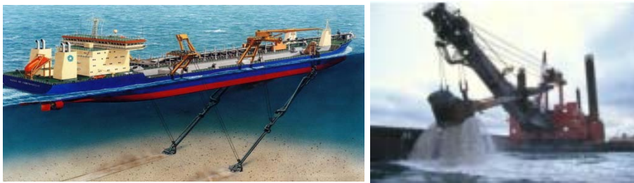
Figure 2.3 Trailing suction hopper dredger, Right: Mechanical Dredger
