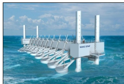
Figure 1.6 Bottom fixed wave power unit Wave Star [6].
