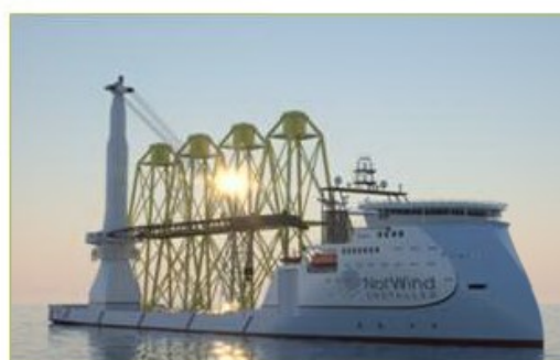
DP construction vessel for jacket installation
