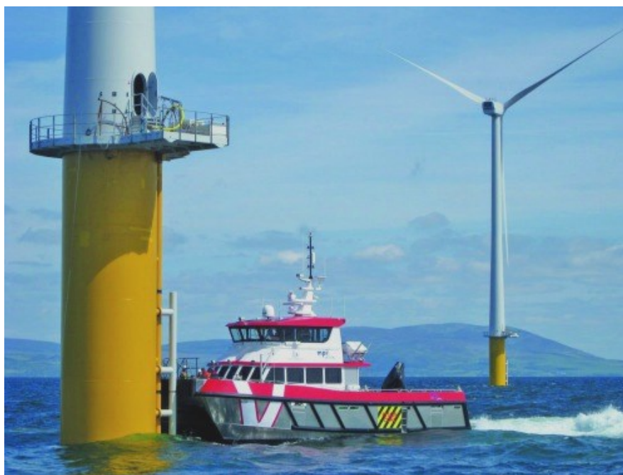
Figure F.1 MPI Don Quixote during a Bow Transfer Operation
