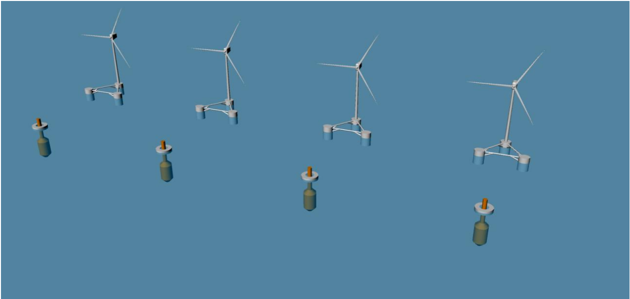
Figure 3.4.4 - Combined wave-wind energy with emphasis on wind energy
