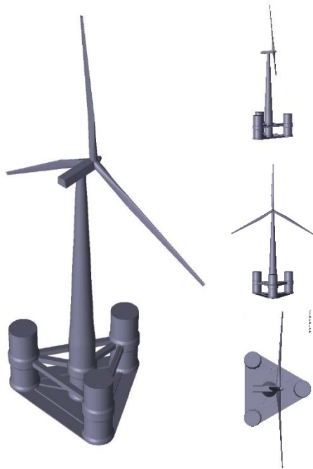
Figure 3 Triangular Semisubmersible Concrete Platform: 5mw Concept Source: Spanish and international patent. Semisubmersible platform for use in the open sea. PCT/ES2013/000165. WO2014/013098A1. UC-FIHAC. Guanche et al (2014).
