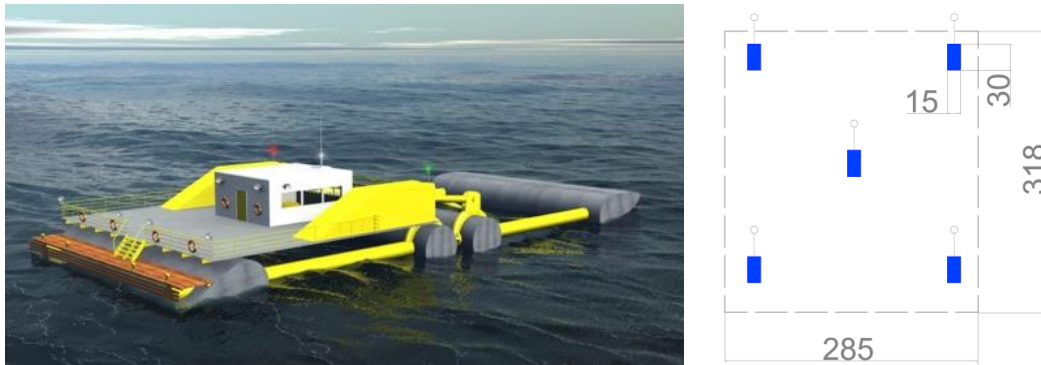
Figure 8-4 DEXA concept (left); proposed module layout with five staggered devices, measures are in meters (right).
