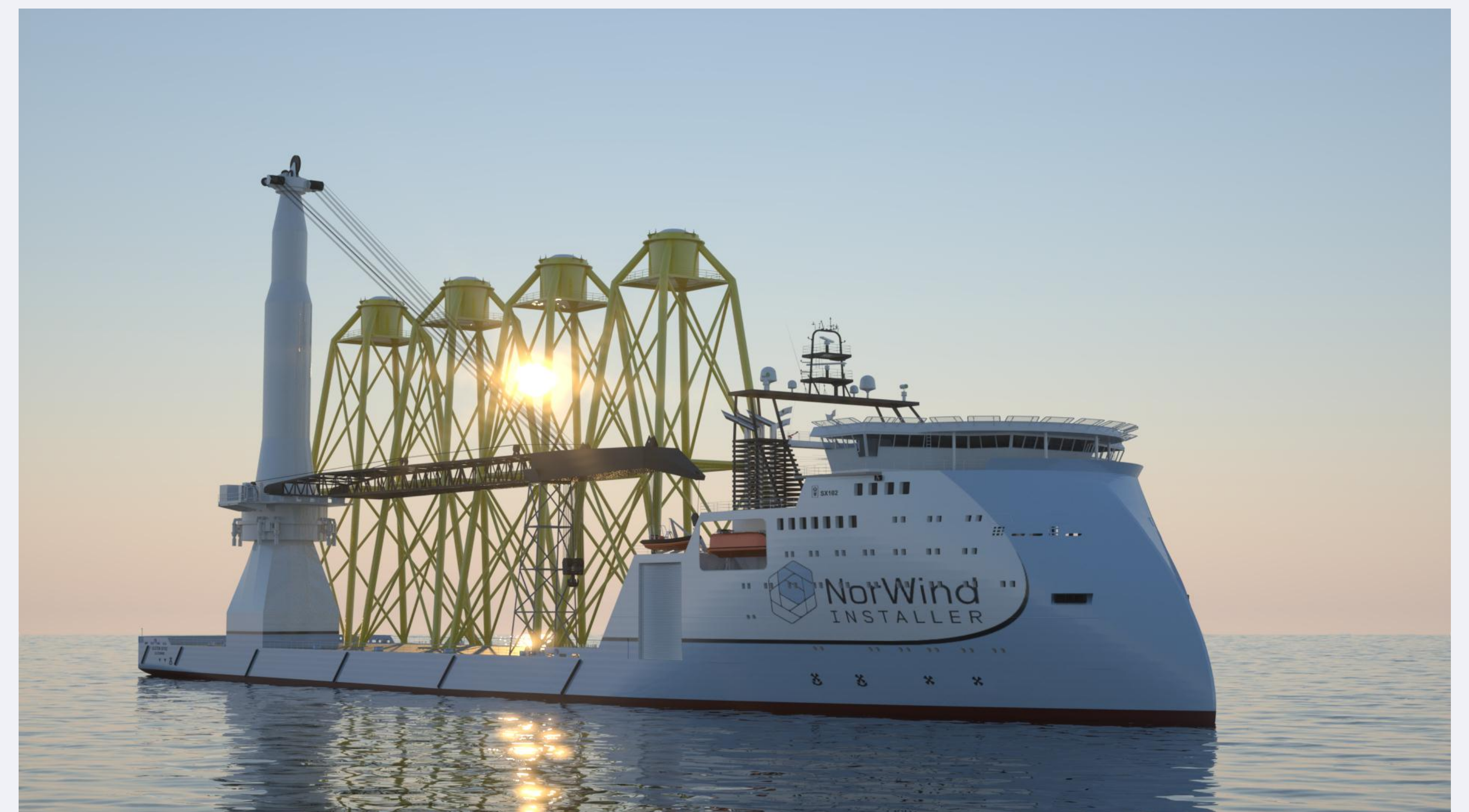
Fig. 2 A new installation vessel for 10 MW wind turbine foundation installation (courtesy NorWind / Ulstein)
