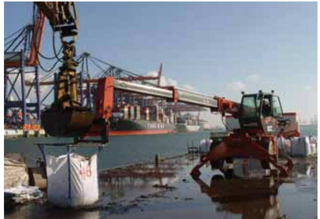
Fig. 2.22. The Manitou, a crane with a long hydraulic jib, moved the bulk bags to the back of the pontoon moored alongside the Triton .
