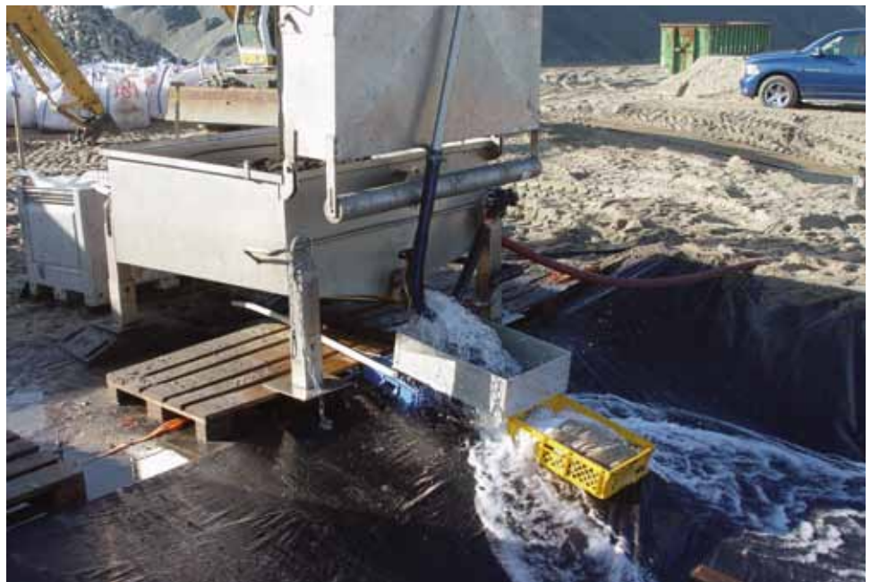
Fig. 2.27. A second, smaller sieve with a 2mm mesh size was placed at the rinse water outlet of the 'Lutter' sieve.
