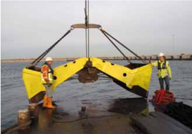
Fig. 2.15. The horizontal level-cut clamshell grab, with a 2 x 5m footprint in open position, that was used during the invasive underwater investigation.
