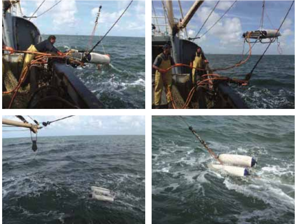
Figure 3. Launching the Boomer from the trawler's starboard side. Photos: Wiersma and Mesdag 2013, 5.
