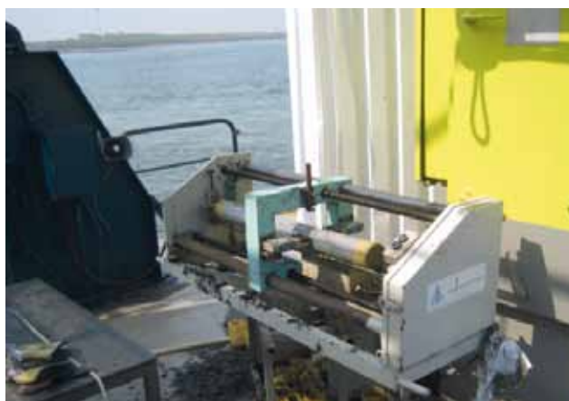
Fig. 2.8. On board the crane ship, the obtained soil cores were cut into 1m segments.
