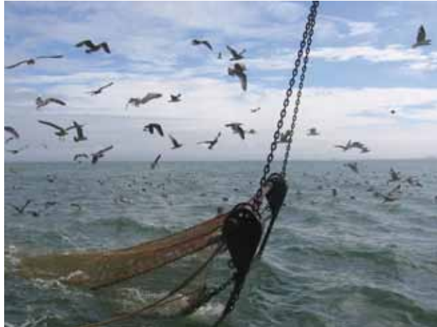
Figure 6. During each transect in the sand extraction zone, beam trawls were lowered on both sides of the vessel to collect archaeological and palaeontological objects from the seafloor. Photo: M. Kuitems.
