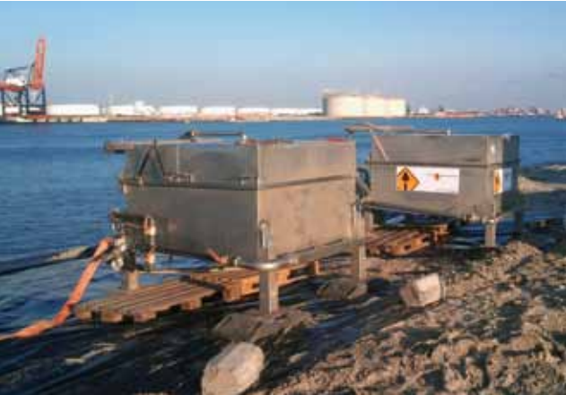
Fig. 2.25. The contents of the bulk bags were sieved using two large 'Lutter' sieves with a mesh size of 10mm.
