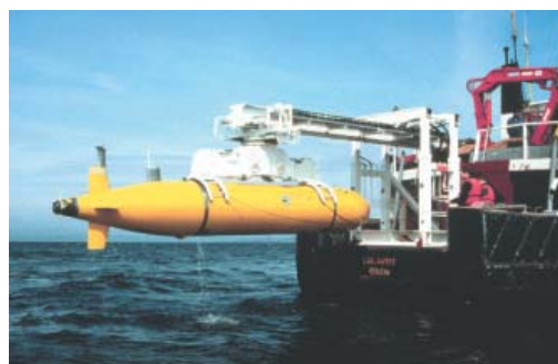
Recovery of AUTOSUB AUV from trials in Scottish sealoch using the RV Calanus . To date, AUTOSUB has achieved 240 autonomous missions with total track of 4600km without support ship control. © SOC Southampton, UK
