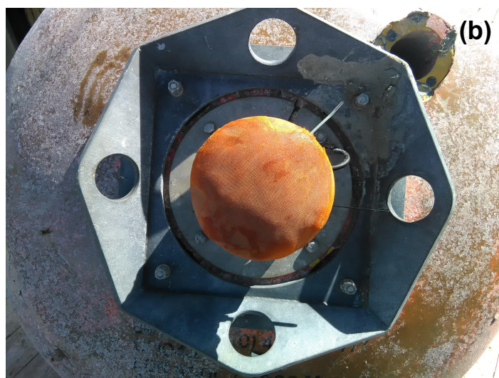
Figure 41: (a) AWAC frame covered with the mixture of udder cream and cayenne pepper. (b) Same as (a), but the mixture is now protected by a pantyhose fabric.
