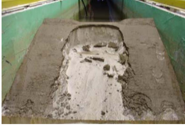
Figure 2-7 Model after breach test (Geisenhainer & Kortenhaus, 2006)
