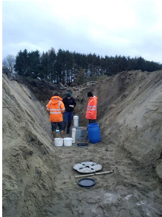
Figure 4-3 Double ring infiltration test in pilot channel
