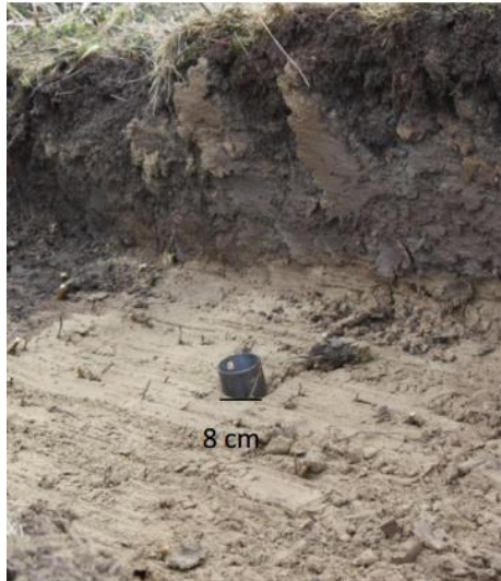
Figure 1-4 clay lining and inner sand core (Irstea, 2015)
