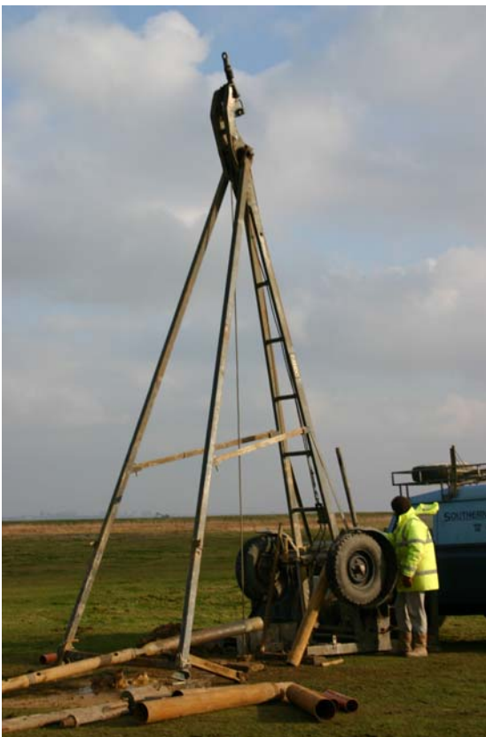
Fig. 3.3.6 Shell and auger survey, Binney Farm, Hoo, Kent (photo: M. Bates)
