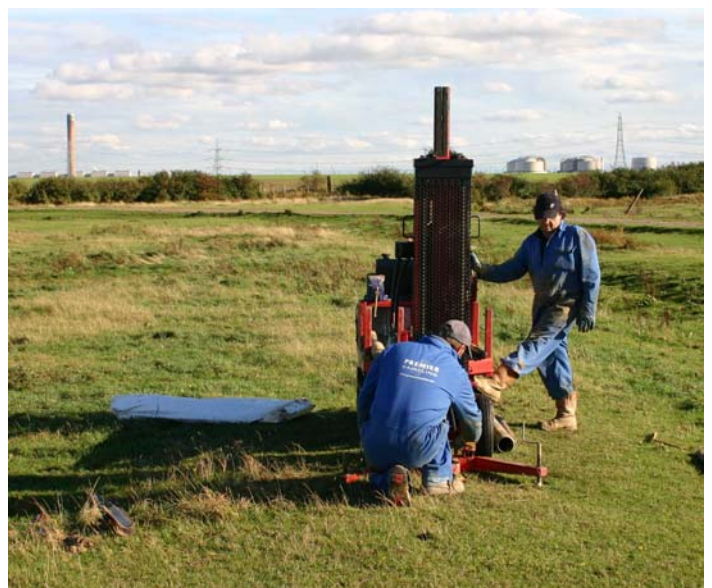
Fig. 3.3.7 Terrier drilling survey, Binney Farm, Hoo Kent (photo: M. Bates)
