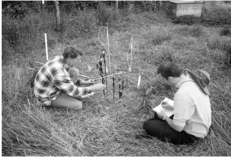
Fig 3.4.4 Recording a redox profile, using equipment developed during the ROB Degradation of the Soil Archive Programme (Senter project 2003/2004, TSA02102: A. Smit/A. Beeker).
