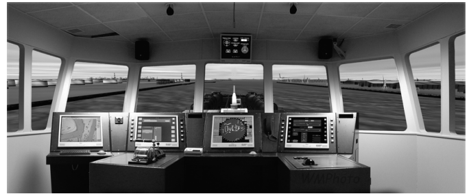
Figure 3 Full Mission Bridge Simulator at Flanders Hydraulics Research
