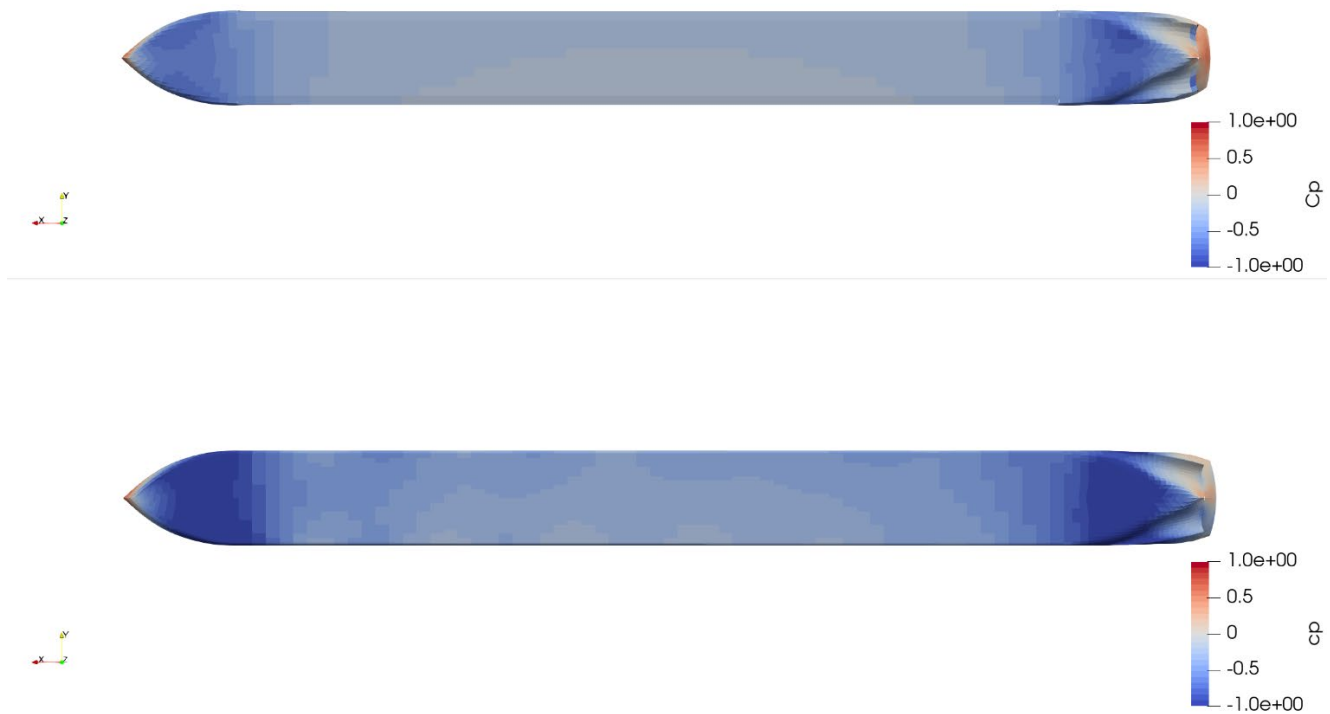
Figure 11. Dynamic pressure coefficient on the appended ship at Flow Interaction (top) and RAPID (bottom)
