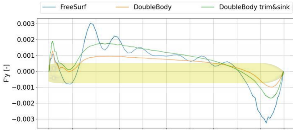
Figure 12. Longitudinal distribution of side force along the ship.
