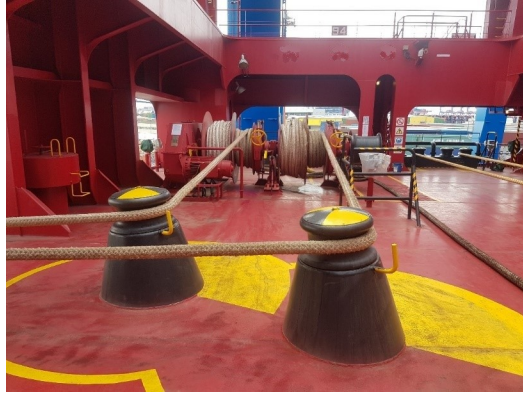
Figure 2.17: Mooring line direction change on deck using rollers, figure courtesy of Hamburg Port Authority.
