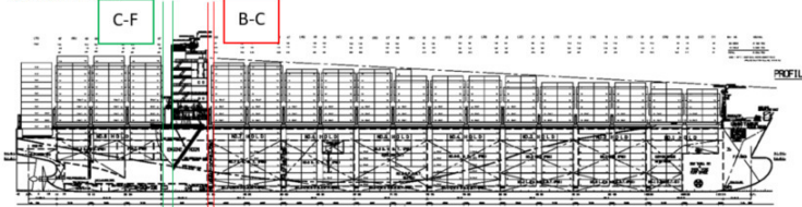
(a) Bridge and engine room not separated, images from RINA Significant Ships of 2014
