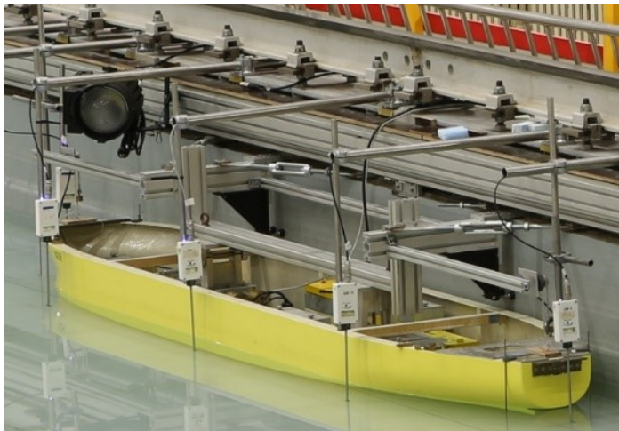
Figure 6.2: Rose Krieger measuring frame for moored ships, example moored T0H.
