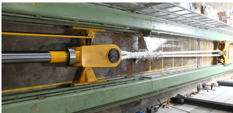
Figure 3.4: Tensile test set-up at Bexco
