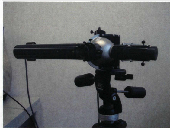
Figure 4: Licor integrating sphere for measuring reflectance and transmittance from filter retained particle samples
