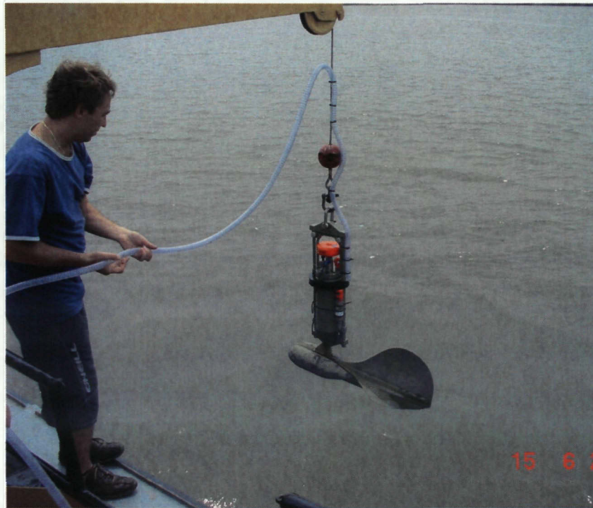
Figure 3: Turbidity sensor with pump installation attached for taking water samples at different depths
