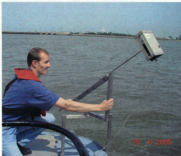
Figure 2: GER-1500 spectrometer measuring downward radiance of skylight at a zenith angle of 40^\circ
