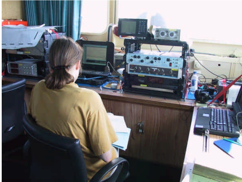
Figure 5: setup of seismic acquisition equipment (single channel surface and multichannel deetow system) on the bridge of R/V Belgica.
