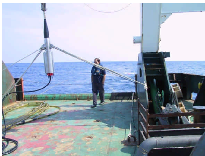
Figure 4: deeptow bottle and multichannel streamer.
