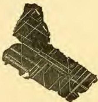
FIG. 14.—Feldspathic basalt of Tristan da Cunha. Opaque section of ilmenite or hematite with cleavages intersecting at 120^\circ .
