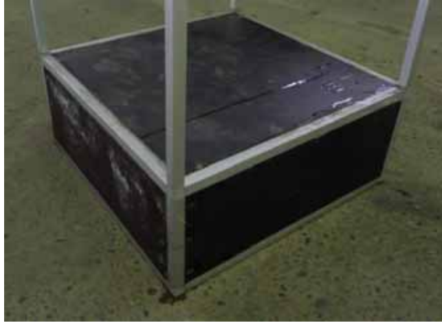
Figure 6.35: A fully reflective obstacle (36 m (w) x 36 m (l) x 15 m (h) on scale 1/50)
