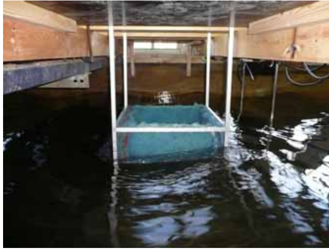
Figure 6.46: Side view of the WEC (36 m (w) x 36 m (l) x 15 m (h) on scale 1/50) in the wave flume of Flanders Hydraulics Research
