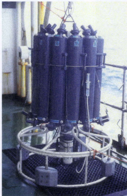
Figure 2.11 Niskin- bottles for water sampling attached to a carousel which also contains the SCTD-probes for measuring different physico-chemical parameters.
