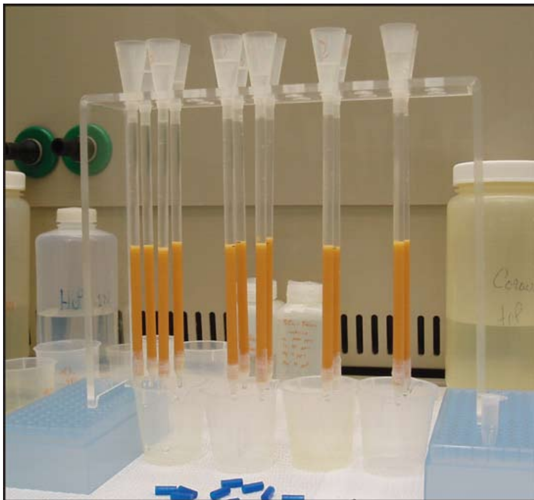
Fig. 2.11 The columns containing AG50X8-resin that are used for the separation of strontium (Sr) and the rare earth elements (REE).
