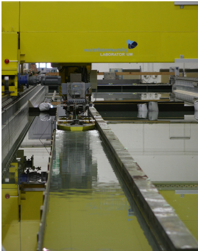
Fig. 2. The KVLCC2 towed in the most confined canal section ( W=1.05 B ).
