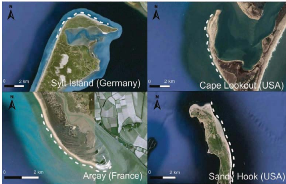
Figure 2: Examples of shoreline undulations observed in Sylt Island Spit, Germany; Cape Lookout Spit, North Carolina, USA; Arçay Spit, France; and Sandy Hook Spit, USA [Courtesy of Google Earth].
