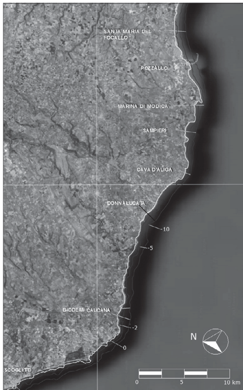
Figure 5: Location of the cross-sections of the beach profile which have been investigated by means of the SBEACH models, by using ETS storm data.
