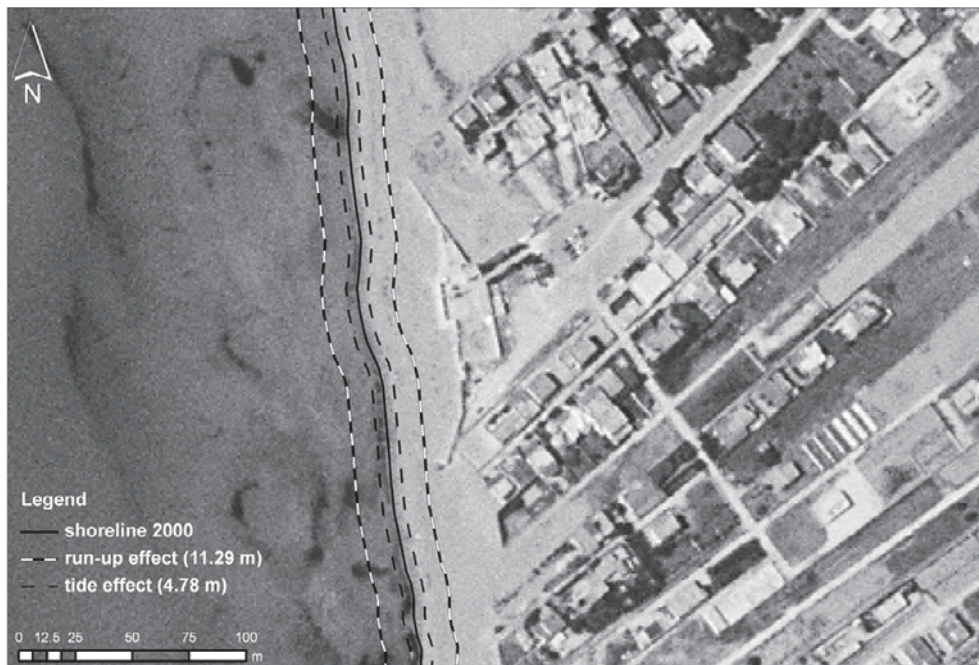
Figure 7: The shoreline strip linked to the ordinary storm (run-up and tide). The total width is about 21.29 m
