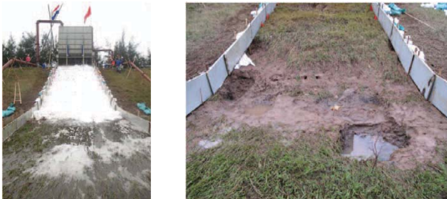
Figure 5: Rough guidance of overtopping flow (left) and damages (right) at dike toe, TL_01.
