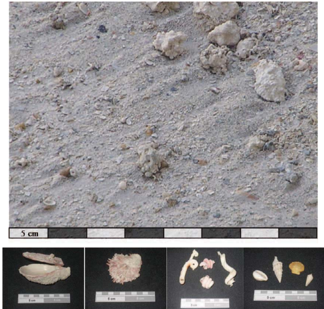
Figure 3: Photographs illustrating the shelly sand composition and the variety of entire shells pumped with the sand
