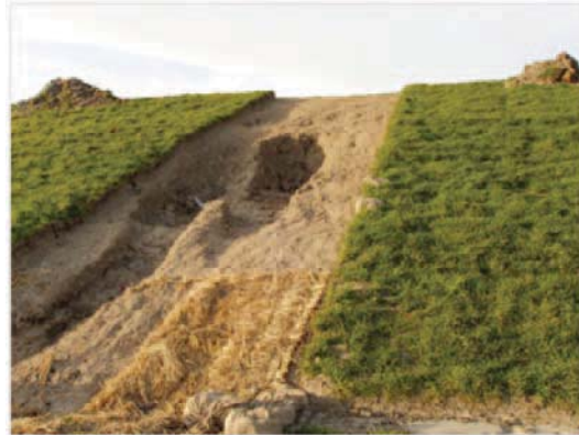
Figure 23: Delfzijl, Groningen, section 3. Bare clay (0.2 m grass cover was removed). Mean discharges of 1; 5; and 10 l/s per m, each during 6 hours. Ongoing erosion during each condition, which resulted in head cut erosion: a horizontal part with a vertical slope; the vertical slope erodes by lumps of clay from the vertical front and the hole increases upwards.
