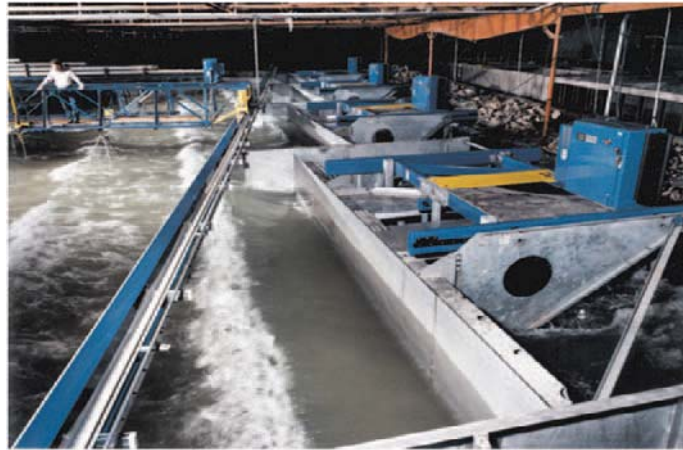
Figure 3: Wave-maker layout in LSTF basin
