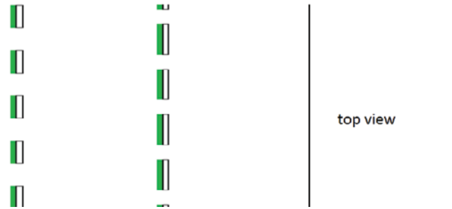
Figure 18: Top view of Figure 17, two open row of walls (with green parapet-nose) creating the stilling wave basin.
