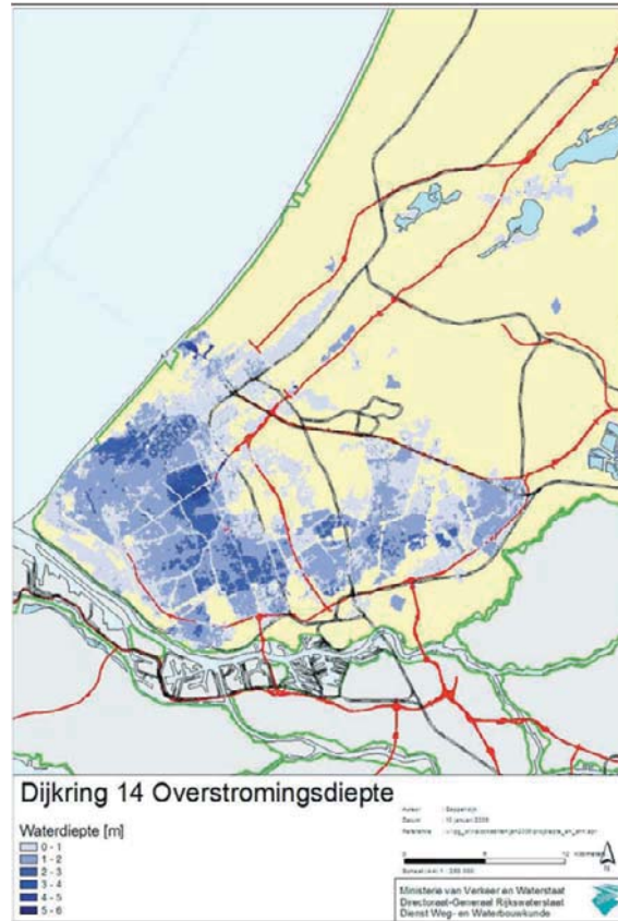
Figure 5: Example of maximum flood inundation depth caused by sea flooding in the Netherlands (EXCIMAP, 2007a).
