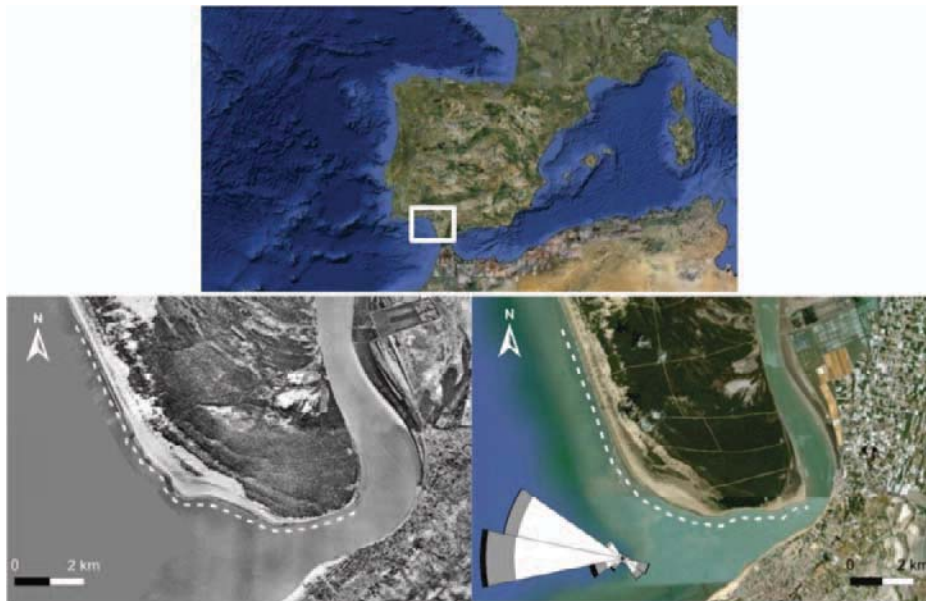
Figure 1: Location and aerial photographs of Doñana spit taken in 1956 (left) and 2008 (right). The shoreline undulations (white dashed line) are present in both photographs. The wave rose of the zone is plotted in the right picture.
