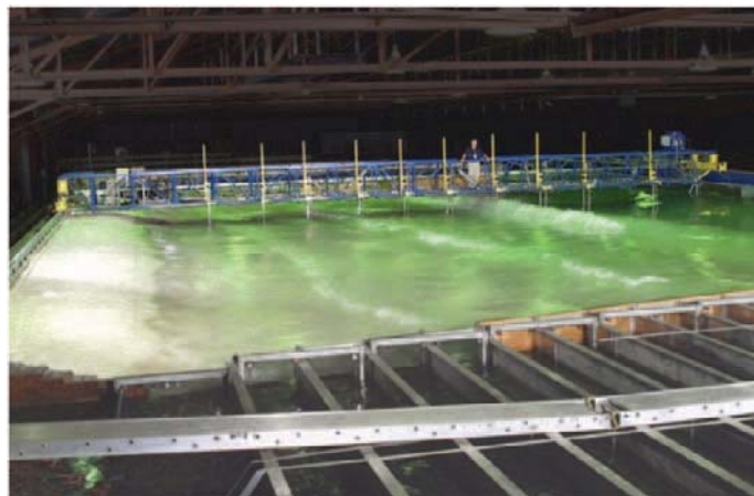
Figure 4: Instrumental bridge and downstream sediment traps
