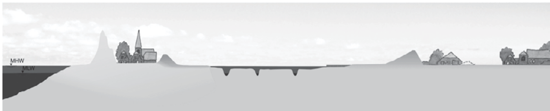
Figure 1: Schematic cross section of coastal defence system "foreland and main dike"
