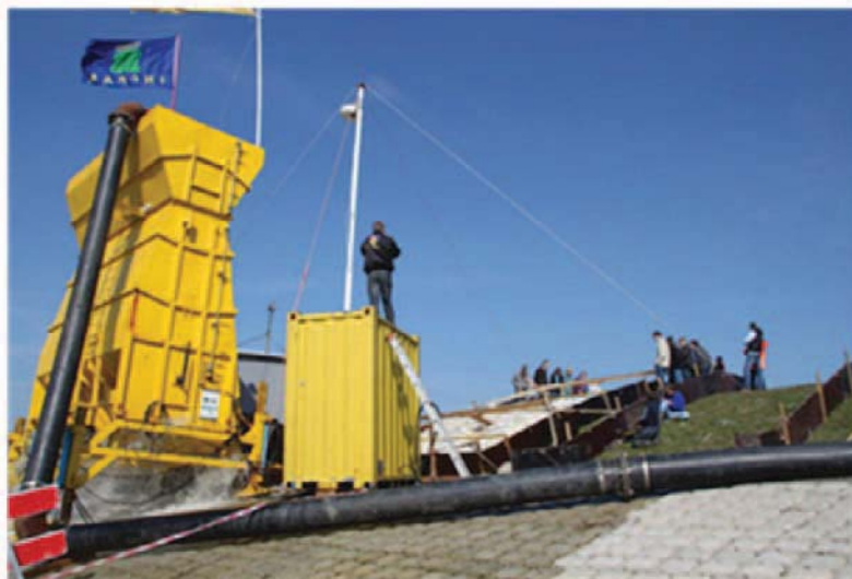
Figure 38: Pilot test on wave run-up simulation
