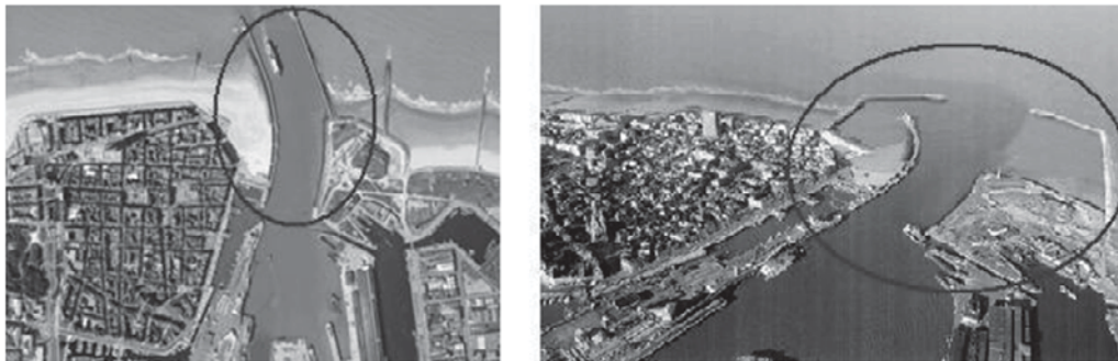
Figure 2: Harbour of Oostende, original harbour dam layout (left), future breakwater layout (right)
