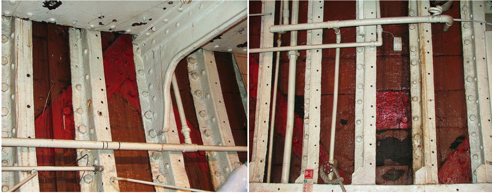
Figure 2: Composite hull structure of the Cutty Shark (Kentley, 2004)
