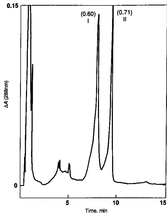
Figure 3 H.p.l.c. of a pyridine extract of indigo powder (for details see text)
