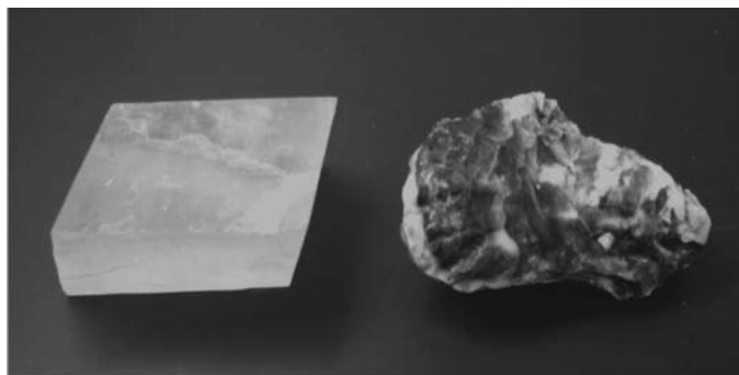
Fig. 6. Naturally obtained calcite (left) and oyster shell (right). Both have same crystal structure, but the apparent features are clearly distinctive.
