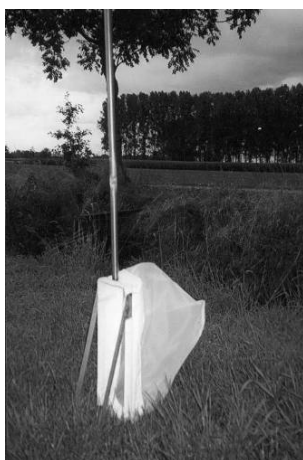
Figure 3: the surber, instrument for sampling macrophytes of 15cmx15cm.
