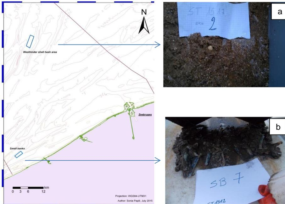
Figure 1: Test areas where Multibeam recordings, video and seabed samples were performed; a) sample with high concentration of shell fragments collected at the Westhinder area; b) accumulation of shells of *Ensis* organism collected at the Small bank area.
