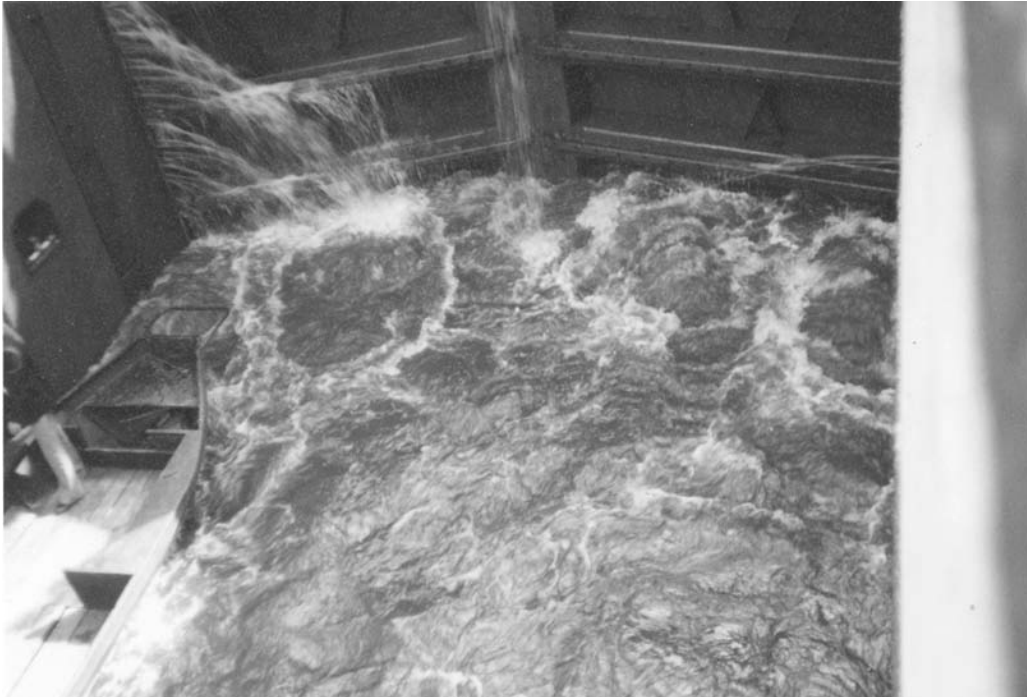
Photo 6.4 Flow pattern during filling by means of gate openings of the lock in the Noord Willemkanaal
