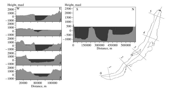
**Fig. 3.** Longitudinal and transverse profiles of Lake Baikal: (0) longitudinal profile from the southern to northern edge of the lake; transverse profiles: (1) across the Southern Basin, (2) at the boundary between the Southern and Central basins (Buguldeika River–Srednyaya Channel), (3) across the Central Basin (Maloe More Strait–Olkhon Island), (4) across the Northern Basin (the Zavorotnyi Cape area), (5) across the Slyudyanskii Cape.
