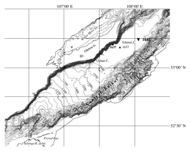
**Fig. 2.** Bathymetry of the Central Basin (a fragment of the computer-based map of Lake Baikal). Isobaths are drawn after 50 m; heavy lines, after 250 m. Isobaths for deep-water zones are numerated starting with 1250 m. Maximum depths of Lake Baikal are designated by black symbols: 1642 m (inverted triangle), based on the computer-based map [3] and GUNIO 1992 map [2]); 1637 m (normal triangle), based on [8]; and 1637 m (box), based on GUNIO 1974 maps [2].
