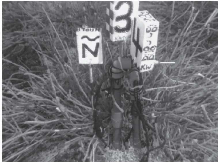
Figure 3. Thermistor array deployed at marker “Ñ” (clump ‘2’). Two thermistors are buried at the base of the clump and the two top thermistors are located at plume level.
