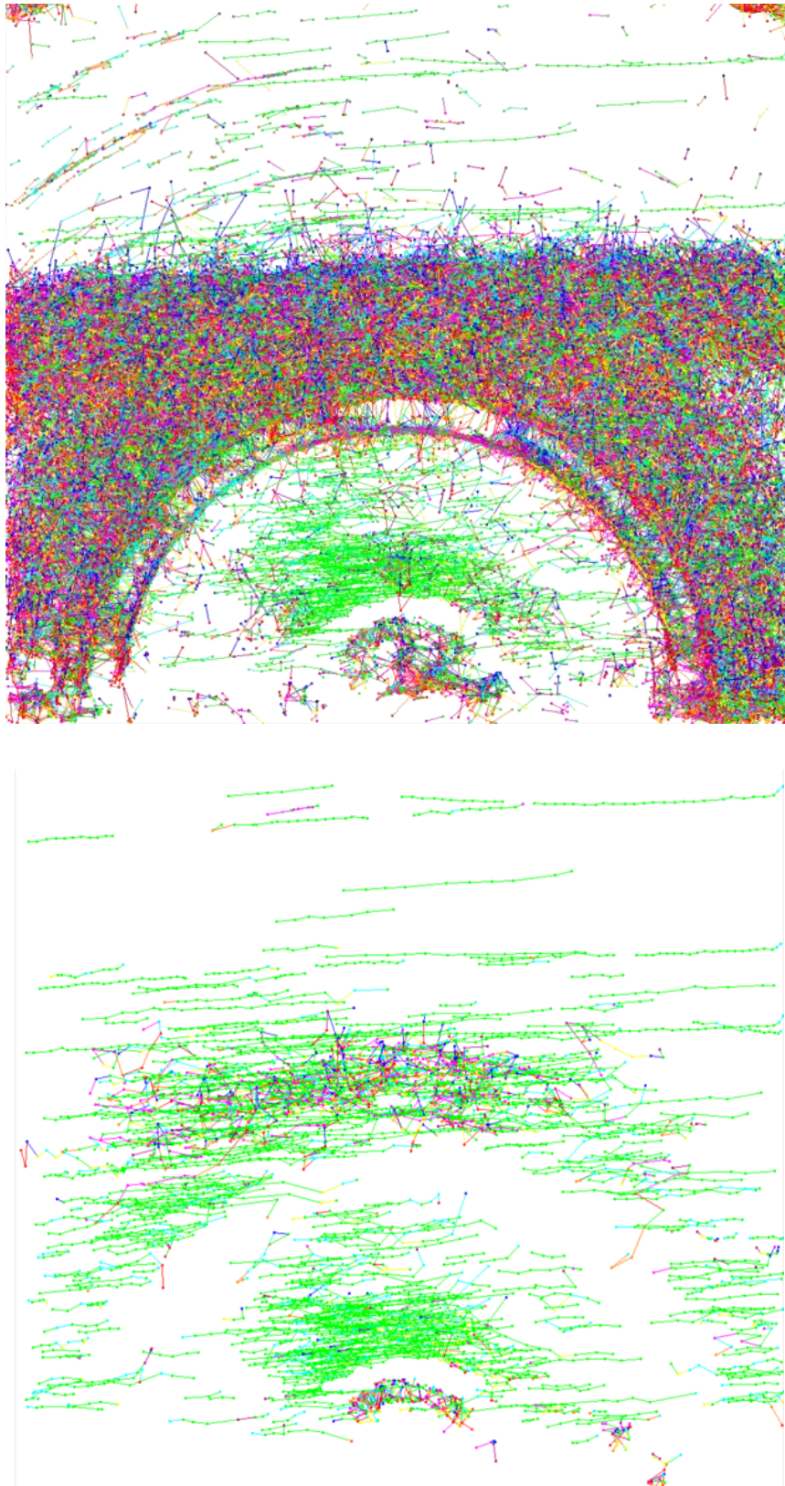
Figure 3. Visualisation of the vertical radar data of April 17 th 2014, before and after the implementation of the decision tree models. Top image shows all tracks registered by the vertical radar, the image below shows the tracks which are classified by the model as birds.
