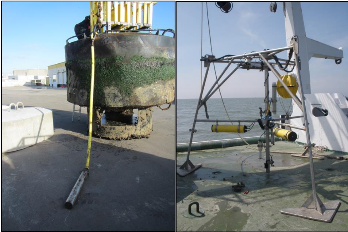
Figure 1. Prevailing mooring systems used: navigational buoy (left) and tripod, in combination with other oceanographic instruments (right) (images: RBINS).
