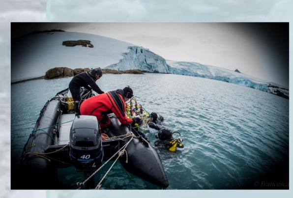
In situ deployment of benthic chambers and sediment profiler with oxygen sensors by skilled divers at 9m water depth
