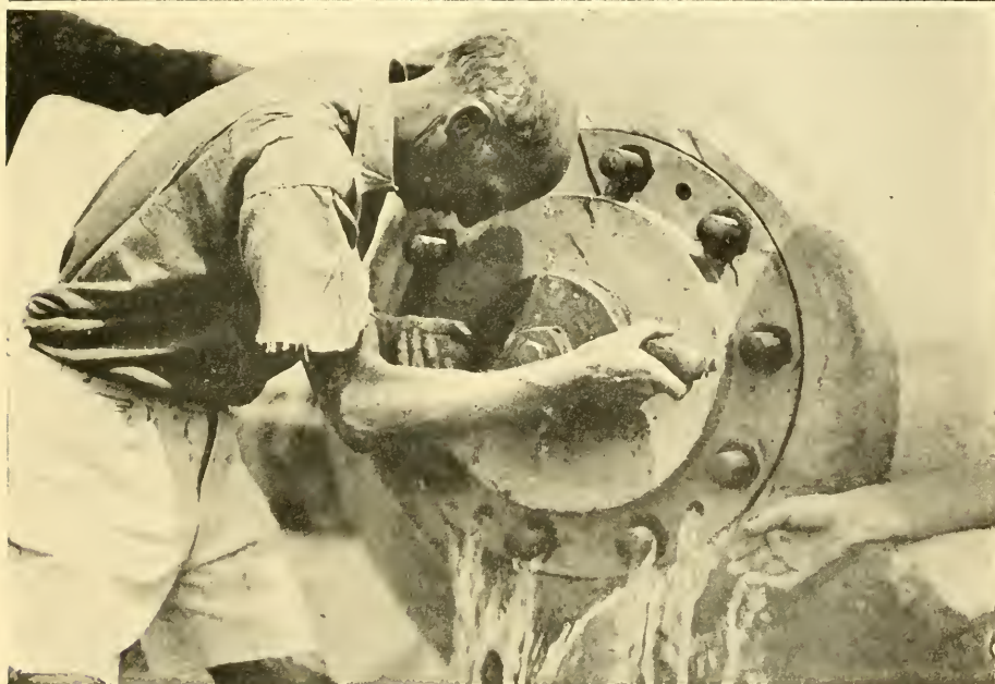
FIG. 73. ( upper ) The central wing-bolt is loosened and slowly turned, and almost at once water begins to drip out, the hissing increasing. FIG. 74. ( lower ) As the wing-bolt turns, more and more water escapes, and the hissing rises to a high scream. On the chance that the pressure might be dangerous, the deck is cleared of people, and the photographer placed far to one side.
