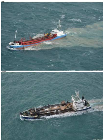
Figure 2: Aerial surveillance: a. A dredging vessel extracting in sector 1a ; b. Fully loaded dredging vessel returning from sector 1a
