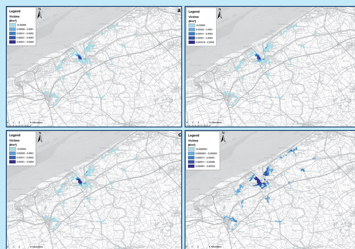
Figure 2 – Spatial distribution of expected number of victims in Nieuwpoort, resulting from the +8m TAW superstorm event, showing that different classification techniques lead to spatial variation of the map content (a: based on equal intervals, b: based on Jenks Index, c: based on standard deviation and d: based on geometrical intervals) Background: Topographic Map of Belgium, 1:100.000, 1986-1990 (NGI/OC GIS Vlaanderen) Source: Vanpoucke et al. (2009), own processing
