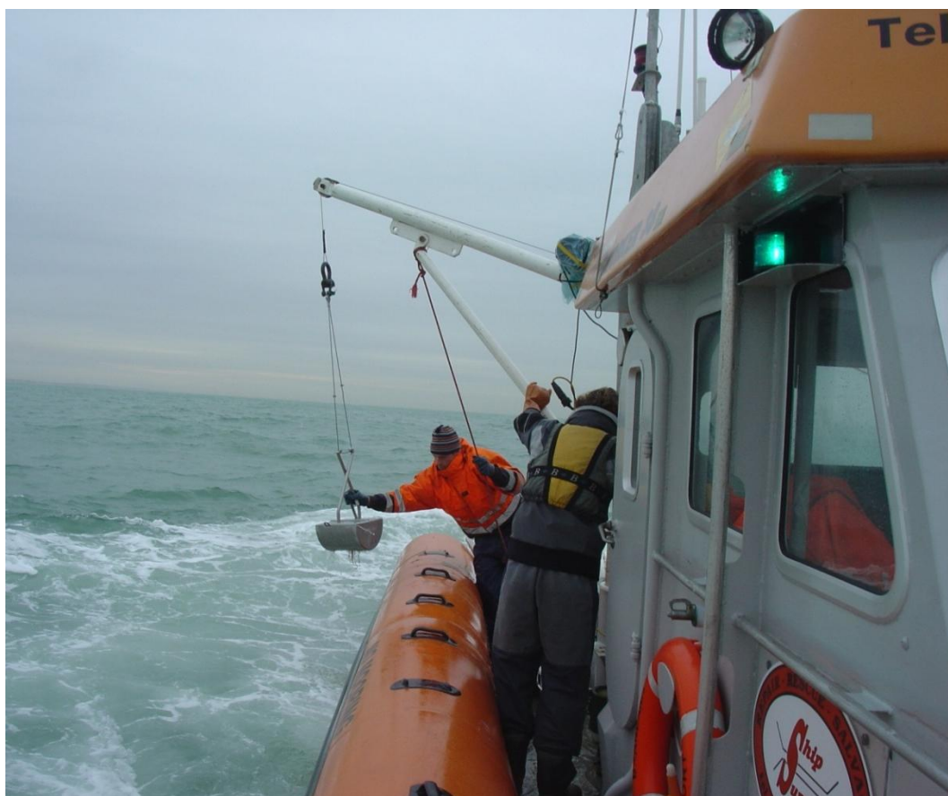
Figure 8.1 The 'Brandaris' has a length of 8.92 m and is 3.40 m wide. The motor of the ship has 500 Pk.
