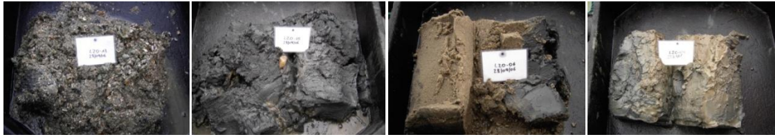
Figure 7.19 High variation in sediment composition, ranging from almost pure shell fragments to very fine mud
