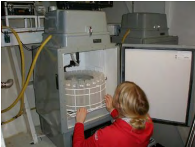
Figure 3.9. An automated water-sampling device, which is part of a Ferrybox-system in the Baltic Sea. Photo: B. Karlson.
