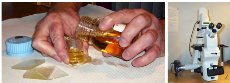
Figure 3.15. The Utermöhl method for settling and counting algae. Left: concentration of samples using sedimentation chambers; right: an inverted microscope. Photos: Å. Edler, B. Karlson.
