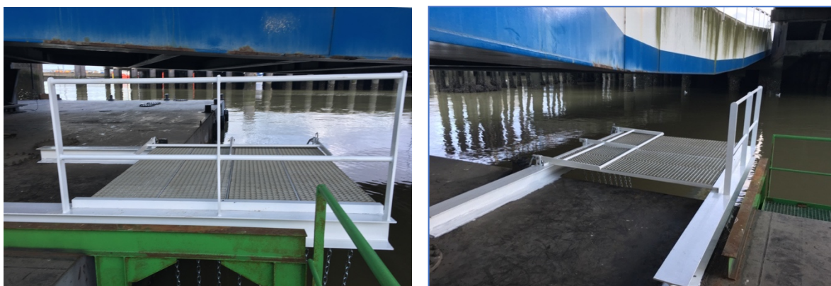
Photographs: new construction for immersion of towing tank test plates for 287 days.
