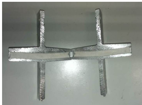
Figure 4: The deformation of the salt core in a casting experiment.
