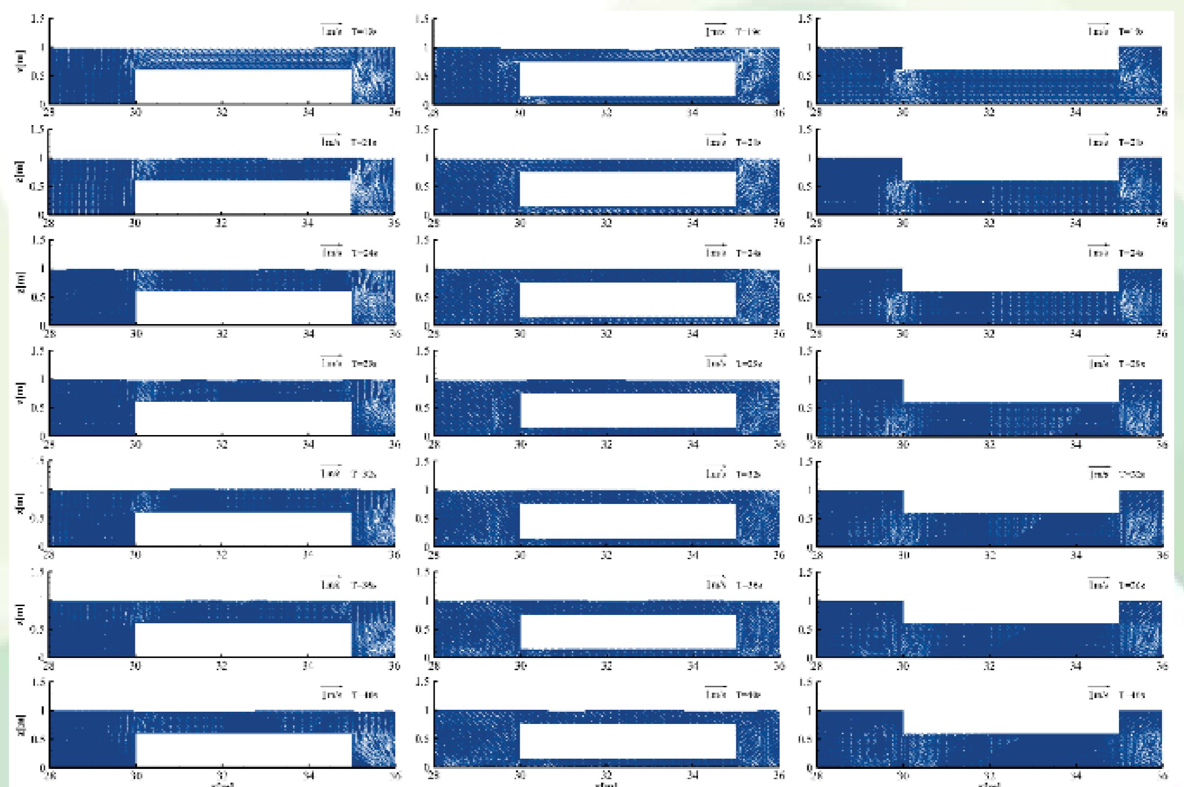
Figure 3 Temporal and spatial variations for the velocity field calculated using numerical mode (left panel: submerged; middle panel: immersed; right panel: floating)
