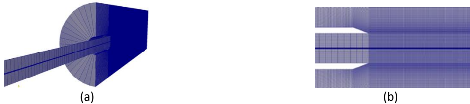
Figure 2 Details of mesh arrangement. (a) Overall mesh arrangement. (b) Local mesh around the nozzle exit
