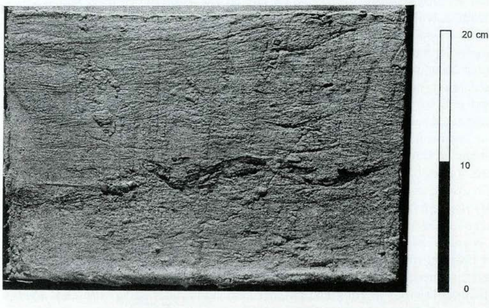
Figure 3.18 Lacquer peel of box core j (Fig. 3.15) showing small-scale cross-bedding of various orientations and intercalated mud flasers. A parallel-laminated set occurs almost at the top of the sequence. The presence and thickness of parallel-laminated sets is considerably less than in core d (Fig. 3.17). Box core from the upper point bar of a tidal channel, water depth about 3 m below NAP. See also Fig. 3.15.
