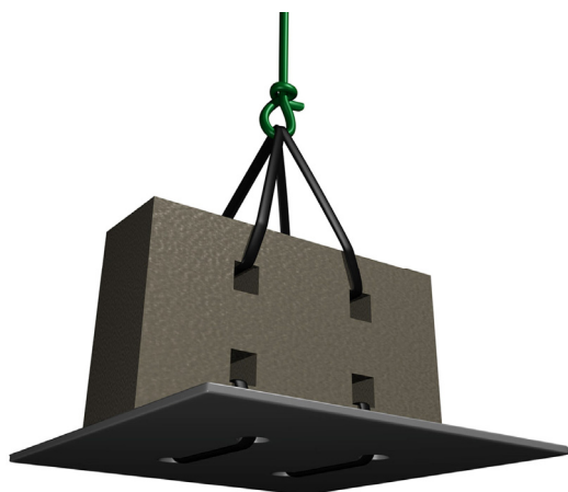
Figure 3. Fouling community plate. The PVC plate measures 14×14 cm and is roughened on the underside. It is deployed at a depth of 1 m.
