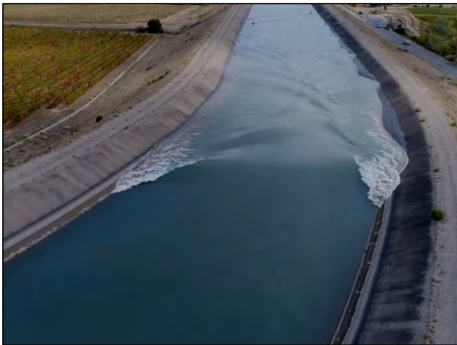
Fig. 18 Wavefront and Favre waves in Manosque headrace canal (test D6)
