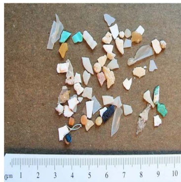
Fig. 2. Images of sampled dry microplastic debris from the North Atlantic Ocean separated into different size classes. The sampling setup in bottom right panel shows a Lambertian Spectralon panel and the aggregated particles on a black rubber background used to obtain a bulk reflectance measurement.
