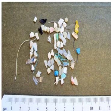
Fig. 2. Images of sampled dry microplastic debris from the North Atlantic Ocean separated into different size classes. The sampling setup in bottom right panel shows a Lambertian Spectralon panel and the aggregated particles on a black rubber background used to obtain a bulk reflectance measurement.
