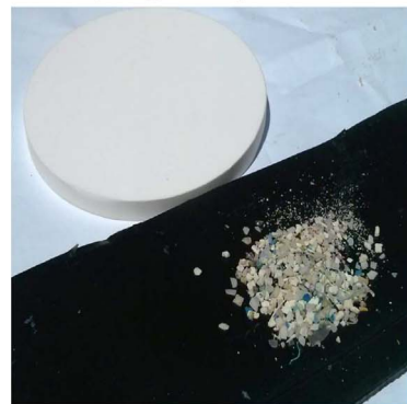
Fig. 2. Images of sampled dry microplastic debris from the North Atlantic Ocean separated into different size classes. The sampling setup in bottom right panel shows a Lambertian Spectralon panel and the aggregated particles on a black rubber background used to obtain a bulk reflectance measurement.
