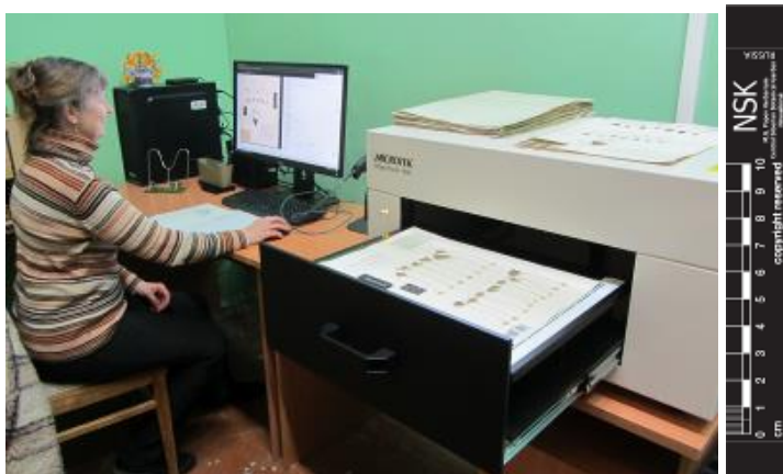
Figure 8. I.Deyun scans herbarium specimens of NSK collections using ObjectScan 1600. 8a. The scale bar. Photos by Nataliya Kovtonyuk
