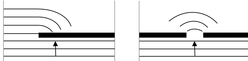
Figure 3.7: Wave diffraction behind semi-infinitely long obstacles
