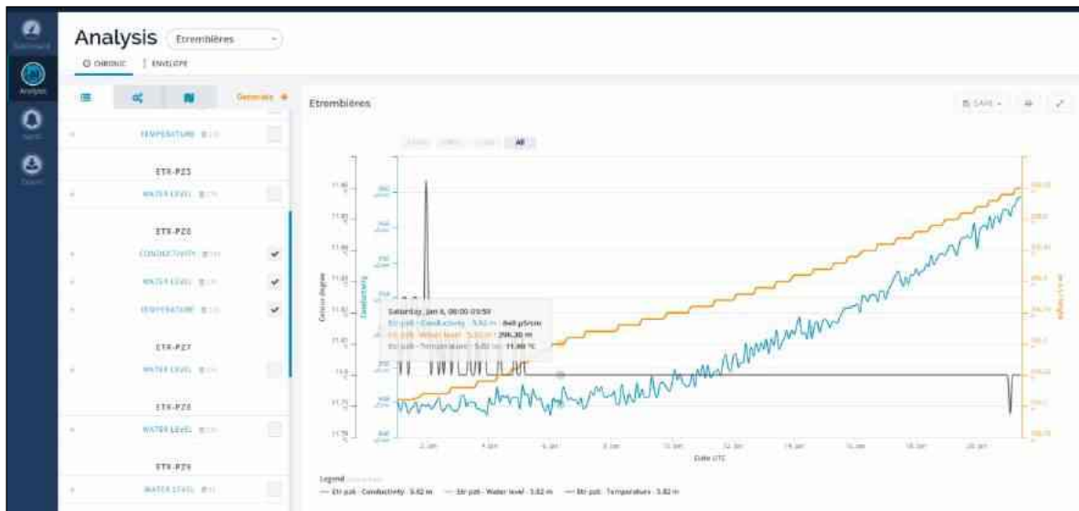
Figure 4: Mutli-parameters curves displaying on the same graph with different colours and scales depending of the parameter (black: T°, blue: conductivity, orange: water level).
