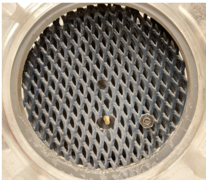
Figure 5.30: Ions precipitation at the cathode surface at high pH value.
