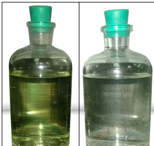
Figure 5.20: Chlorine evidence collected from the anodic electrolyte: (left) after the experiment, (right) the same solution after few weeks.
