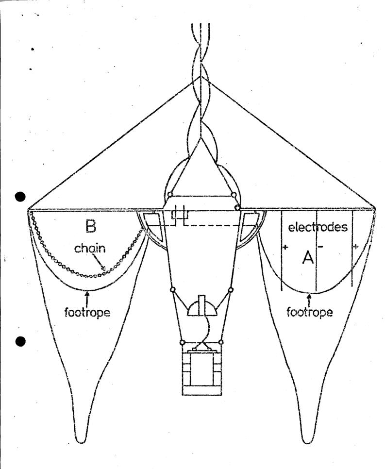
Fig 1. Schematic diagram of towed sledge and nets.
