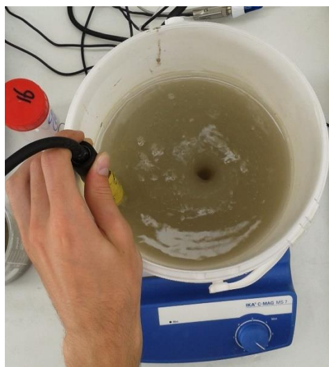
Figure C1. The bucket with the water being stirred by the magnetic stirrer (not pictured, on the bottom of the bucket) and an OBS.
