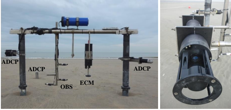
Figure 48. Left: The intertidal measuring frame (1 m high, 2.2 m wide) with the down-looking ADCP, up-looking ADCP (not on the frame), three OBS, ECM, and up-looking ADCP. Right: the LISST
