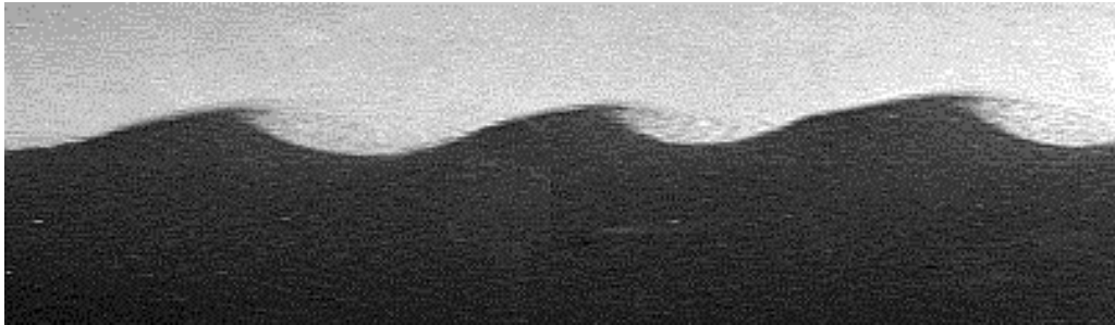
Fig. 4: Video image (15cm long) of the sediment surface for a high inclination angle ( \alpha = 50^\circ ) and large flow rate ( Re_p = 15 )
